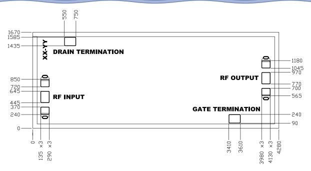
Overall die size 4280 x 1670 (+0/-50) microns, die thickness 100 (+/-10) micron. All Gate and Drain pads must be wire bonded for electrical connection.
